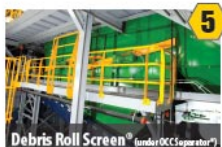
Debris Roll Screen® (under OCC Separator) Removes fines, including glass, from paper and containers
