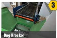
Bag Breaker Opens bags without damaging material
