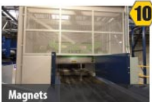
Magnets Captures ferrous metals
