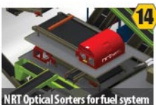
NRT Optical Sorters for fuel system Removes PVC & metals from low quality paper & non-recyclable plastics to create ReEngineered Feedstock™
