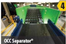
OCC Separator® Separates cardboard from paper, containers and fines
