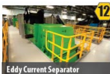
Eddy Current Separator Captures aluminum cans from material stream
