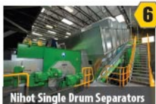
Nihot Single Drum Separators Separates heavier material from lighter, high-value recyclables
