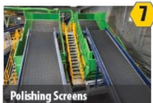
Polishing Screens Separates into 3 streams: mixed paper, containers, fines
