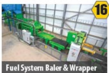
Fuel System Baler & Wrapper Compresses ReEngineered Feedstock™ into wrapped bales for final product
