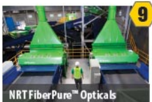
NRT FiberPure™ Opticals Optically detects and ejects plastic film from mixed paper
