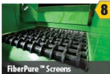
FiberPure™ Screens Removes small contaminants from mixed paper
